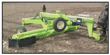
"The perfect companions to the Schulte 2500 "Giant" are the Schulte models SRW 1400 and SRW 800 Windrowers. These units windrow scattered rock from 2"-25" diameter, into neat rows. This greatly reduces the time required to clear rock and debris from the field.
